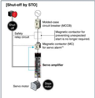
Figure 2: Possibilities exist by utilizing softwarebased safety, in this case, STO safety subfunction. (Source: Mitsubishi Electric)
