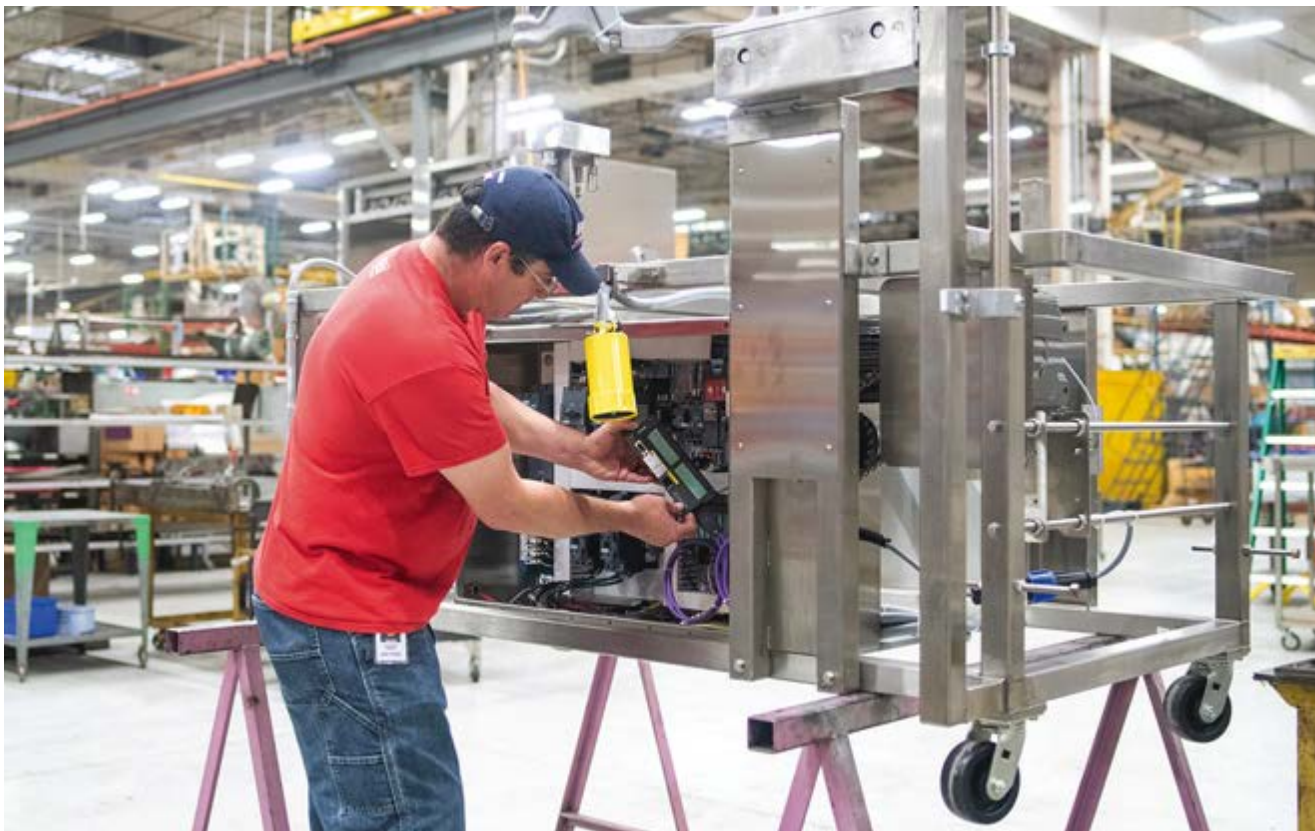
Figure 2: John Priddy, Krispy Kreme fabrication manager, installs the newly developed kit into the fryer section of a doughnut machine.
