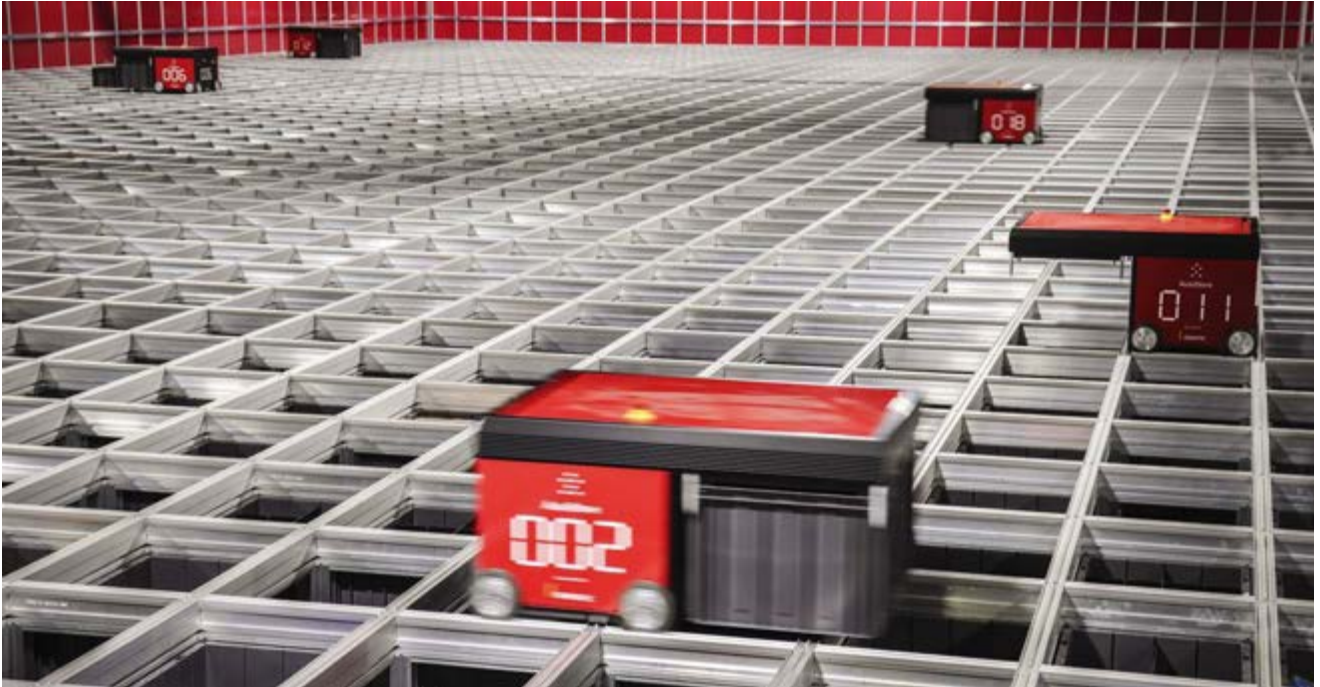
Figure 1: An automated goods-to-service system is key to maximizing productivity in this Motion distribution center in Birmingham, Alabama. (Source: Motion)
