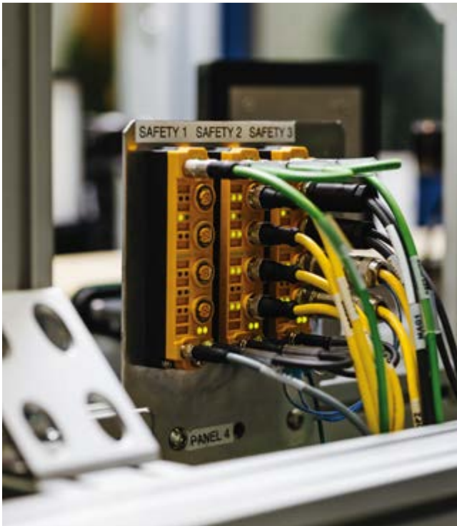
Figure 2: Machine-mountable safety solutions provide robust options for functional safety. (SOURCE: BECKHOFF AUTOMATION)
