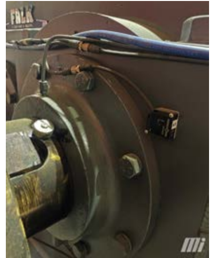
Figure 1: This gearbox is enabled with Industrial-Internet-of-Things (IIoT) monitors for vibration, temperature, speed, oil level and oil condition. (SOURCE: MOTION)
