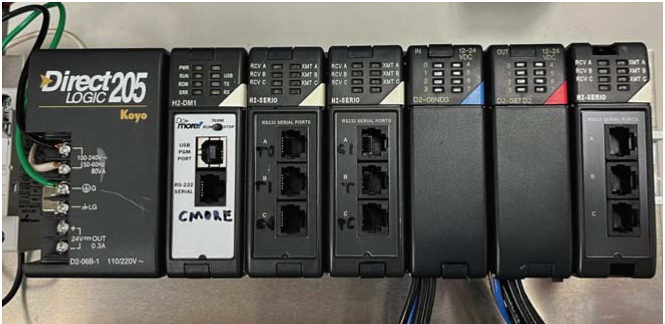
Figure 1: The chassis includes three H2-Serio modules, each of which has three RS-232 serial ports. There is an additional serial port available on the CPU, bringing the total available number of serial ports to 10.
