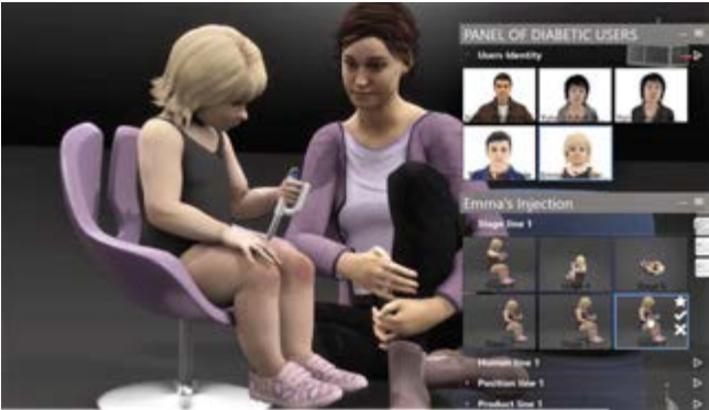
Figure 3: Designers can use a virtual twin of a human body to analyze the sizing and ergonomics of their device and the force required to insert a needle into the skin for various patient types, ranging from adults to children.
