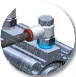
Leakage from piping connections due to poor piping installation
