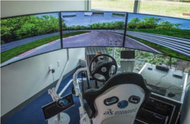
Figure 2: The use of driving simulators can evaluate and improve vehicle handling and control systems in response to changing road conditions and driver reactions.
