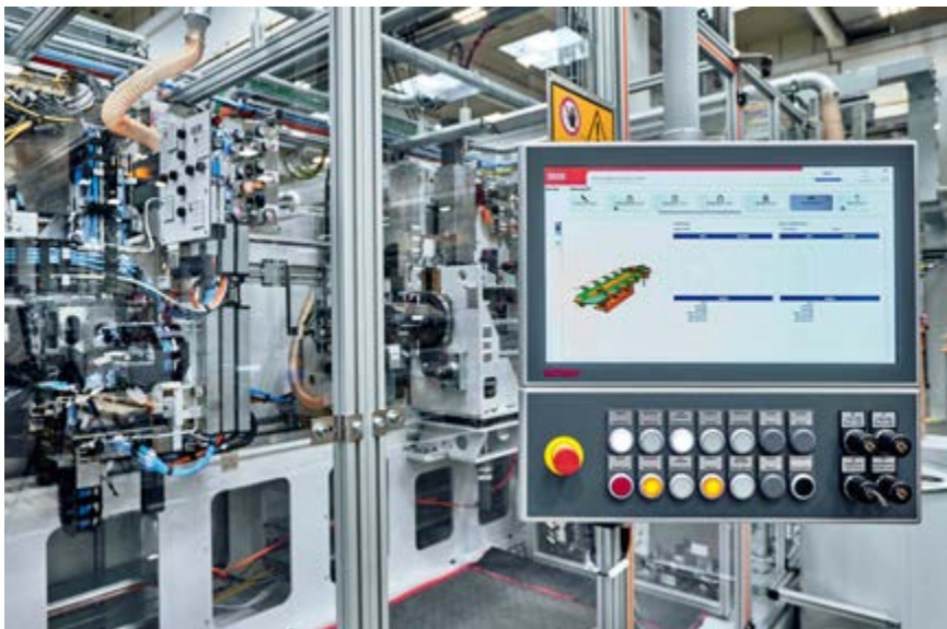
Figure 4: Some PC-based controllers provide a lifecycle of 10 years, plus another 10 years of service. (Source: Beckhoff)
