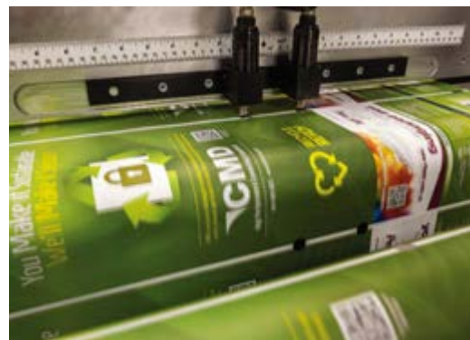
Figure 1: For CMD, EtherCAT simplified the synchronization of a gusset pouch with the continuous material flow. (SOURCE: BECKHOFF)
