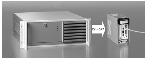
Figure 8: EtherCAT leads to smaller Controllers
