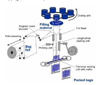
A bag foil is fed via a loop control to the filling station. Because the foil feed is subject to slippage, the exact position of the foil is constantly updated using a register mark encoder. A
