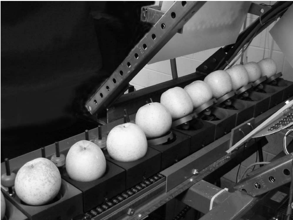
Fig. 3. Conveyor and imaging area. Apples are tilted 45° while they rotate in front of the camera. This is located out of view of the image, outside the upper right hand corner.
