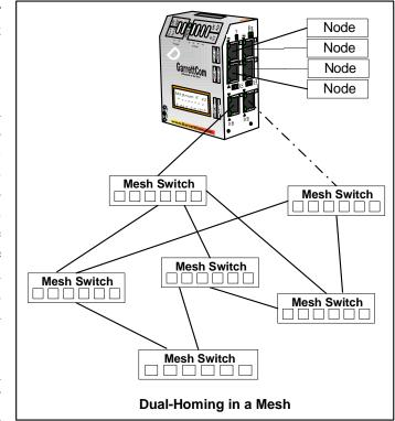
upstream. Media types for ports 1 and 2 may be either copper or fiber, and each port's media type can be configured independent of the other. Additional media types (such as wireless) may be inserted so long as the Link signal is passed through to provide a reliable signal for switchovers between the Operating and Standby Ports of the dual-homing switch.
