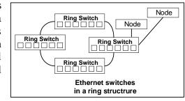
Dual-homing also provides connection flexibility during network maintenance. A switch in the ring may need to be taken out of service temporarily to load new software or to perform a hardware
