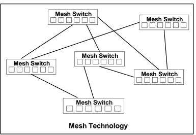
STP or RSTP. The mesh operation will vary the forwarding and blocking ports for the mesh switches as the network goes through changes and recovery from a fault or faults. Exactly how the switches will operate to recover from faults cannot always be predicted or tested. The reliability advantage of the dual-homing switch in a mesh is that it is small, simple, and predictable. Because it is inherently a much more reliable device than the typical managed mesh
