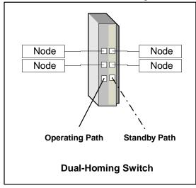
to be connected to the network by way of two independent connection points (points of attachment). One access point is the operating connection, and the other is a standby or back-up connection that is activated in the event of a failure of the operating connection.
