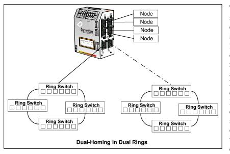
To use this dual-homing switch in a dual-ring LAN, connect Port 1 into any switch in one ring and Port 2 into any switch in the other ring. The same faultrecovery logic in the switch as for single rings is used in handling fault conditions in dual-ring LANs. Loss of Link on the Operating Port causes the dual-homing switch to move all traffic on the upstream connection Standby the Port. to effectively reversing the
