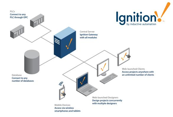
Ignition by Inductive Automation™ is an industrial application server, used to create systems that cover the full spectrum between HMI, SCADA and MES. Its unique architecture enables accessibility from any computer no matter the operating system, rapid project development and deployment, and massive scalability without complexity.
