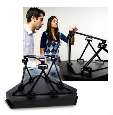
involved the study of kinematic and dynamic simulations of 6 degree of freedom Prismatic-Universal-Spherical (P-U-S) type manipulators. A parallel manipulator combines a platform that moves and a fixed base, interconnected by several legs. In his
