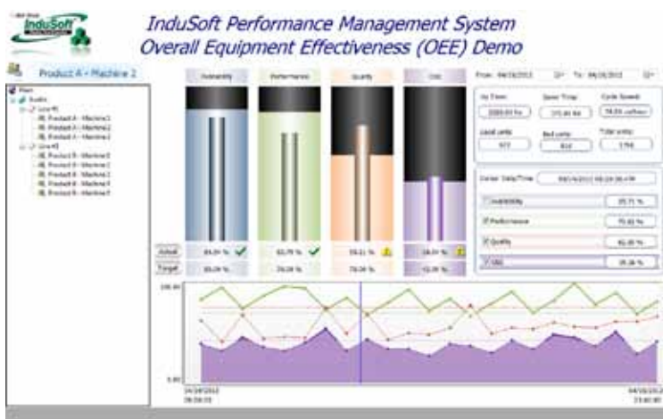
Figure 1: OEE dashboard. Plant managers and executives can now access important OEE measurements remotely to improve quality and efficiency.
