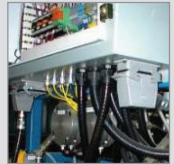
Field assembly time for devices and control cabinets is dramatically shortened using connectors instead of hard-wiring.
