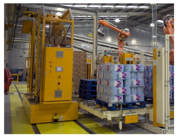
Figure 1: Example with AGV and safety work zones
