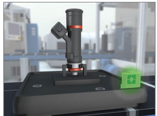
Standard industrial WIP (work-in-progress) applications require hardened RFID tags that can withstand impacts and light liquid exposure.
