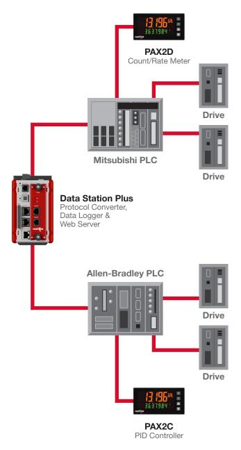
Red Lion's Data Station Plus supports more than 300 industrial protocols to enable disparate devices to communicate seamlessly.
