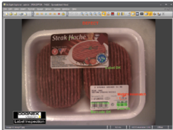
(b) Product label at bottom rejected because actual product weight is .25 kilograms, but listed product weight is .5 kilograms.
