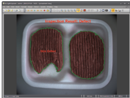
(c) Size defect in meat patties. A consumer typically rejects such a package for being underweight.
