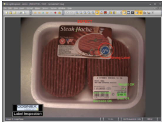
(c) Product label at top rejected because incorrect preprinted labels were installed on the labeling machine. The blue, circular fat content icon shows 0% fat rather than the actual 5% fat, misrepresenting the product to consumers.
