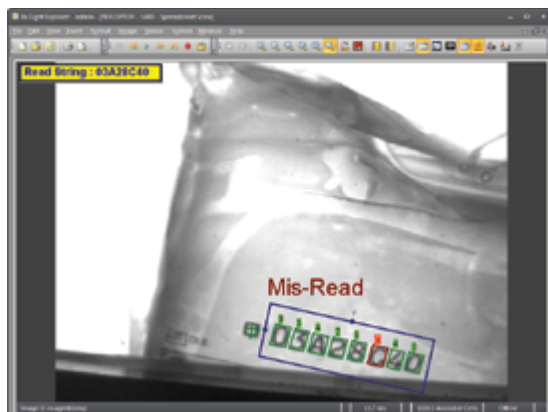
(b) Misread of code caused by misprinting of the letter G, which makes it look more like the letter C. This bag is rejected to avoid confusion.
