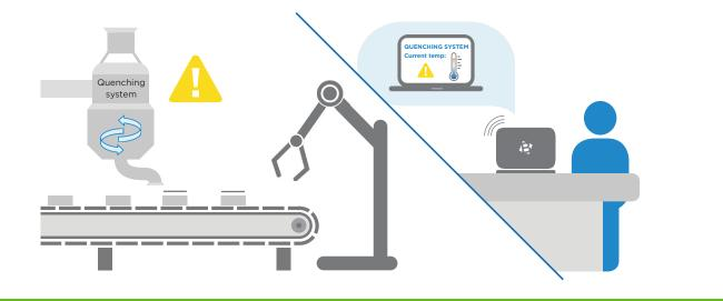
The programmable logic controller (PLC) alerts the lloT solution that thermal couplers have detected rising water temperatures. The solution increases data transmission to 10-second intervals to update the quenching system's digital model, then applies predictive analytics.
