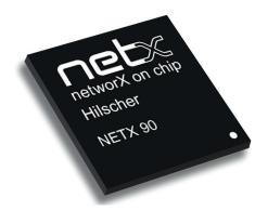
In essence, netX 90 is a powerful slave-to-network gateway solution that supports data communications for motion control, sensors, actuators, encoders, remote IO, and even functional safety devices. It meets the five key requirements listed above and is the first (and only) microcontroller in the market to provide multiprotocol capacity for real-time communications for factory and process automation.
