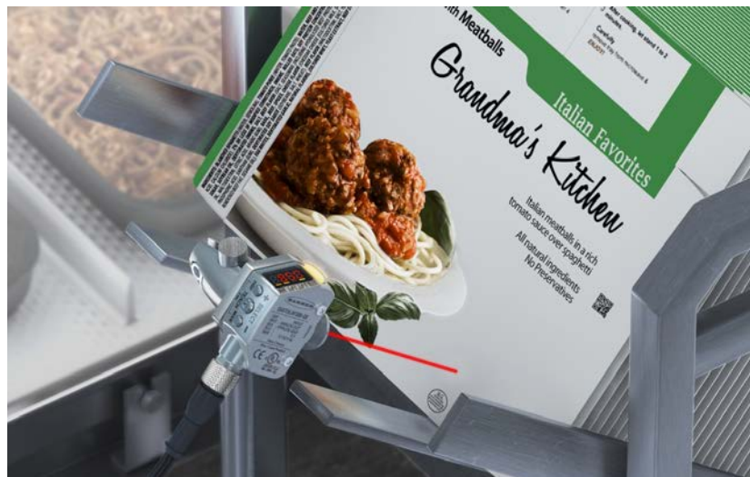
Q4X laser measurement sensor monitors stack height
