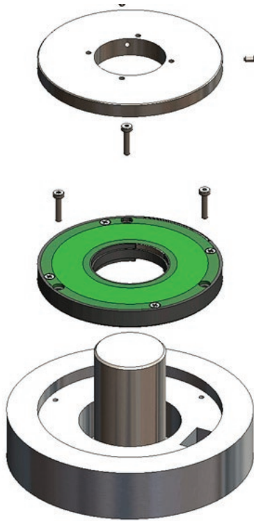
Figure 5: Hollow Shaft Installation
