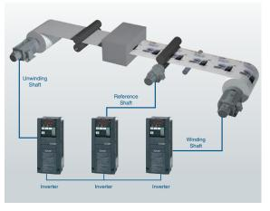
The final mode, which is torque control with load-cell feedback offers the best performance. The system is operating with two control loops. Closing the loop on torque rather than velocity means that tension error scales directly as torque. Meanwhile, the system is also operating on direct tension feedback. This is executed with a PID loop for very accurate trimming.
