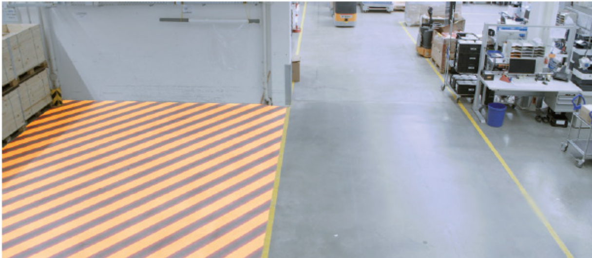
Fig. 6: Predefined geozones can, for example, be goods receiving areas or dispatch lanes.
