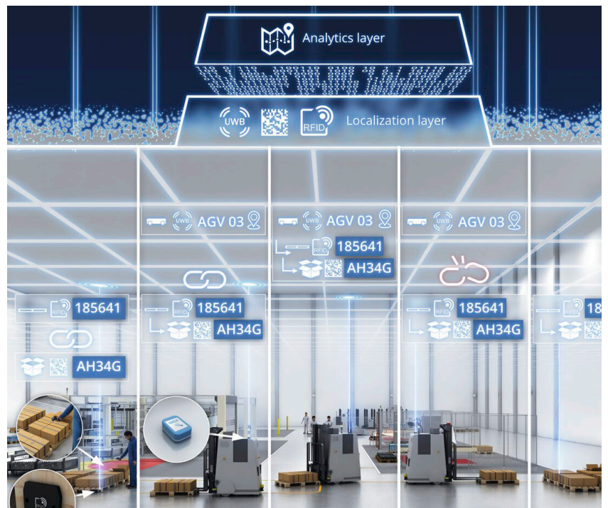
Fig. 9: Indirect localization of high volume, small assets involves linking the identification data of those assets with the location data of larger movable objects, for example manned forklift trucks.
