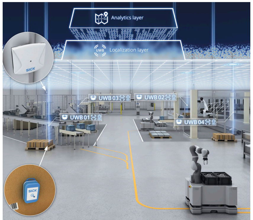
Fig. 8: Determining the absolute location of assets using UWB tags and UWB receiver antennas (LOCU1xx and LOCU2xx from SICK). The data collected can subsequently be visualized, analyzed, and further used in the Asset Analytics platform from SICK.
