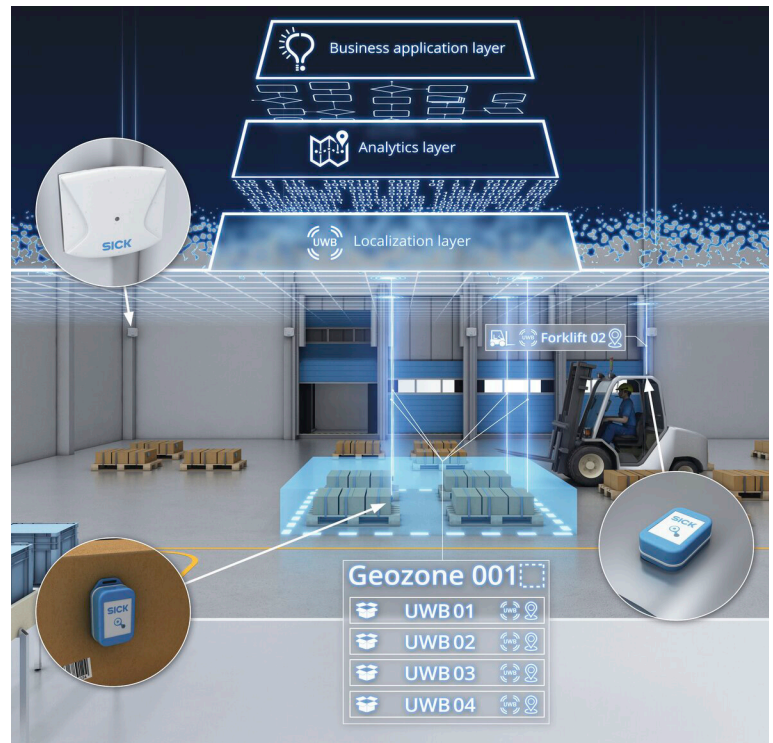
Fig. 10: The data collected in various geozones are forwarded by the Asset Analytics localization software to higher-level ERP systems and MES.
